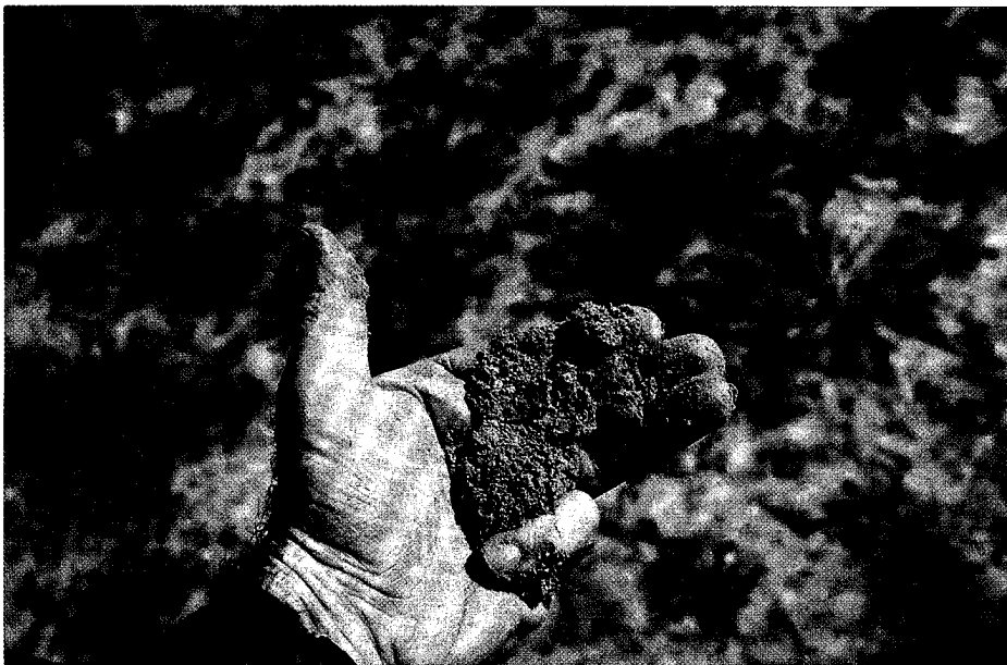
Figure 3.3. A sandy loam textured soil will not form a ribbon when moistened and rubbed between thumb and forefinger.
