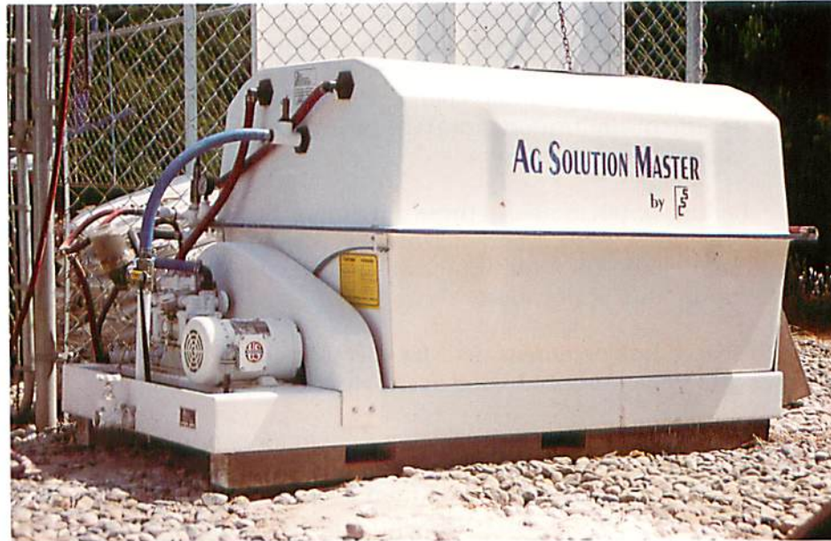
Figure 4.1. Machine for dissolving and injecting gypsum into irrigation water. No endorsement of company named in the picture is intended. Photo credit, Jerry Rivers.
