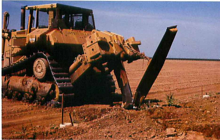
Figure 4.7. Deep tillage with this slip plow can significantly improve water penetration through stratified soils and soils with claypans and hardpans. Photo credit, W. E. Wildman.
