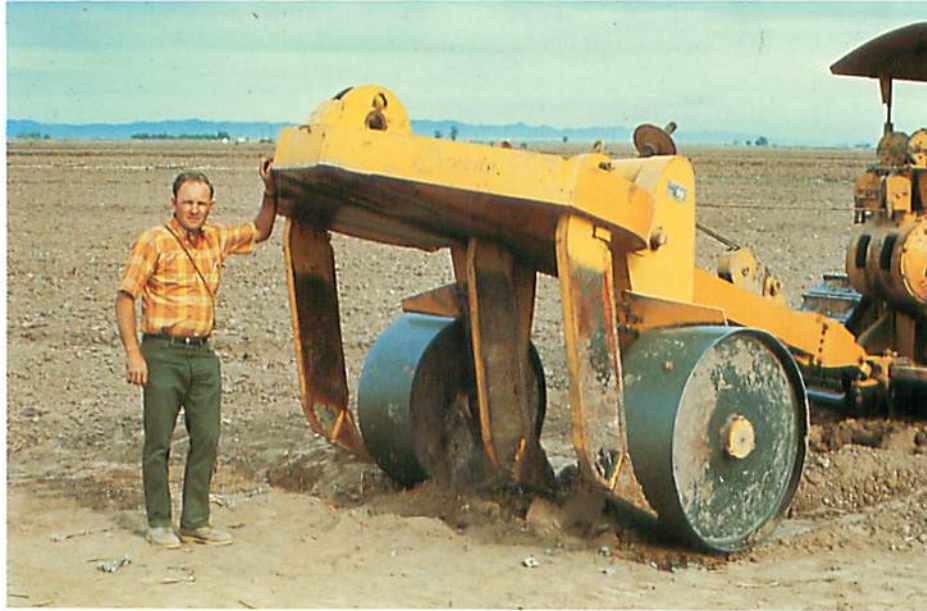
Figure 4.6. These ripper shanks are about 3 feet long and if fully inserted into the soil, will reduce compaction to about 1.5 feet. Photo credit, W. E. Wildman.
